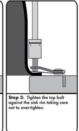
Please note: The countertop is shown upside down in these installation directions, but sinks can be mounted from underneath as well.
